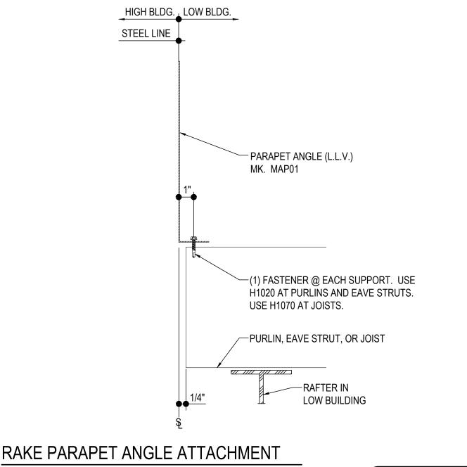
RAKE PARAPET (RAFTER IN LOW BUILDING)
